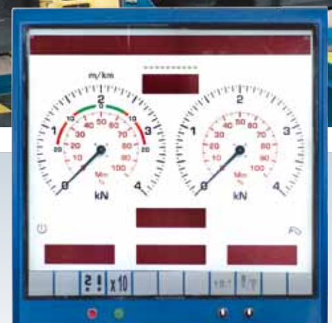
Clearly readable dials, combined with the VARIODATA digital displays and operator prompting (running text) including switch cabinet.
