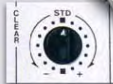
fig. 1: Field adjustment function for fine tuning of the calibration for materials which differ from factory standard calibration material; the displayed value can be increased or decreased in \pm 1.5\% increments
