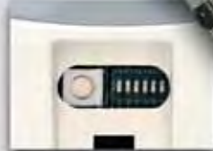
fig. 3: DIP switches for operator settings, such as update rates, memory mode, etc.
