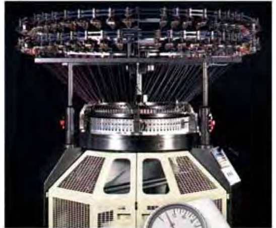
In the Knitting Industry exact adjusting of yarn feeders of circular knitting machines
