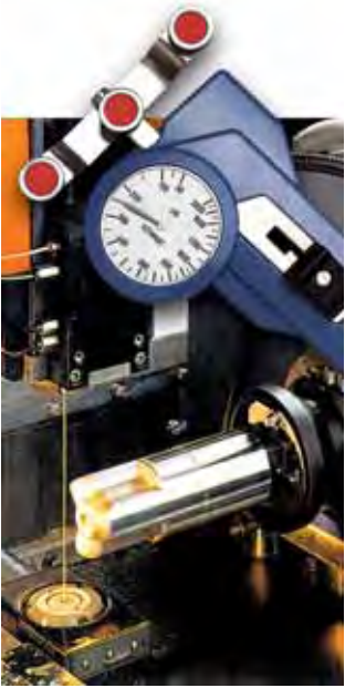
In the Wire EDM Technology the correct adjusted tension is the condition for best exact cuts cutting tools
